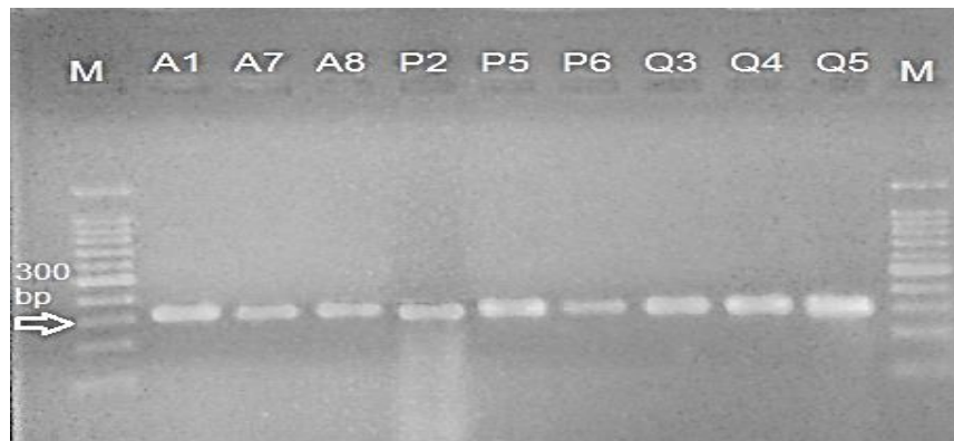
Figure 1- 318 bp bond related to specific planF primer in L. plantarum PCR product electrophoresis was formed. M; 100 bp marker.
